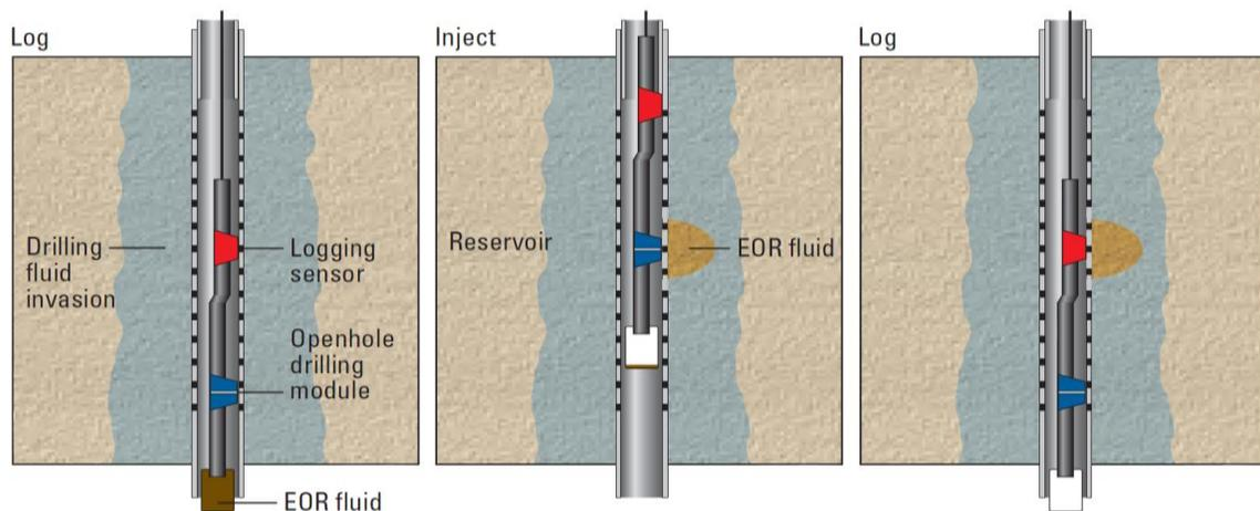
**Figure 1: Schematic of the single-well in situ EOR evaluation procedure. In the first pass (left) the initial saturations are logged, then the EOR fluid is injected (center), and finally the logs are run again to assess the remaining saturation after injection (right). (From Al-Mjeni *et al.*, 2010)**
