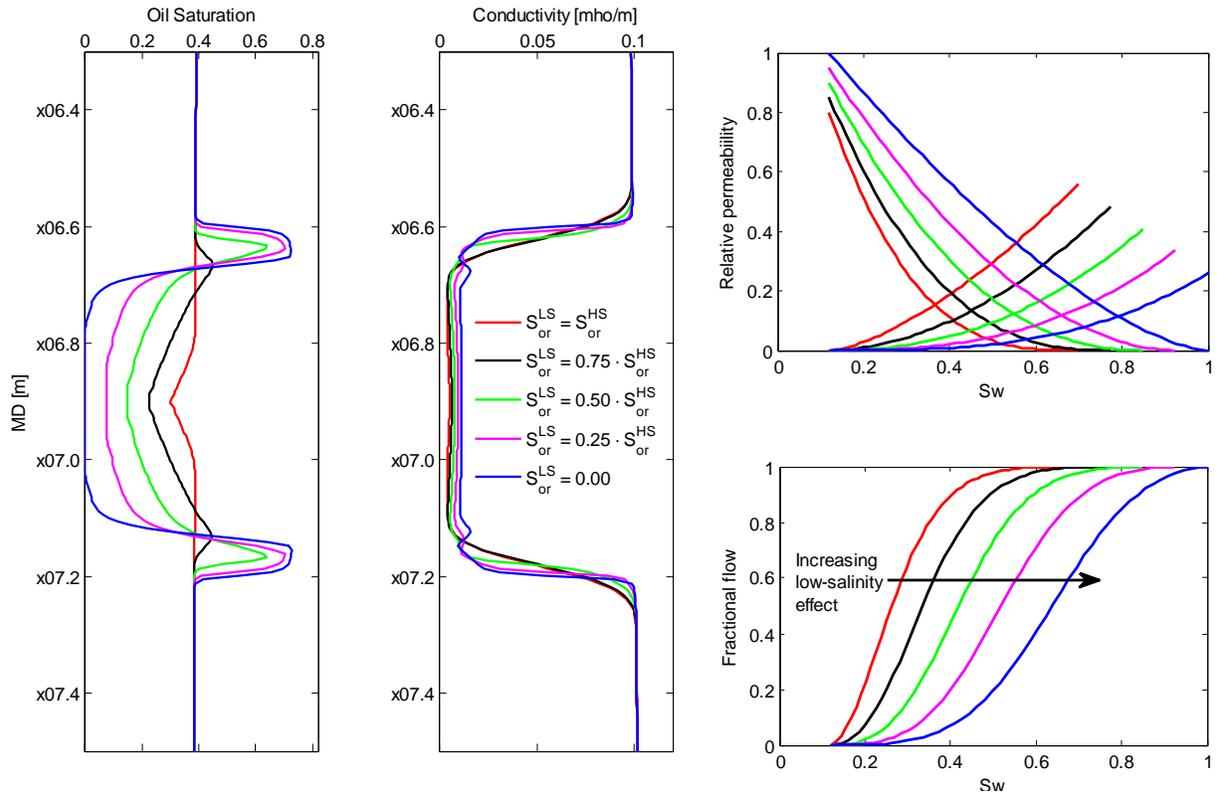
**Figure 9: Simulated oil saturation and conductivity depth logs for low-salinity brine injection. Results are shown at varying degrees of low-salinity effect. The relative permeability and fractional curves are shown to the right. The base high-salinity curves are shown in red.**
