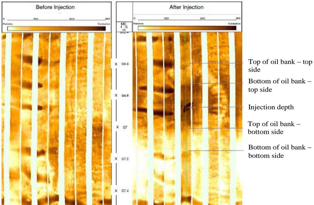
Figure 2: Test 1: Comparison of electrical borehole images before and after ASP injection. (From Arora *et al.*, 2010)
