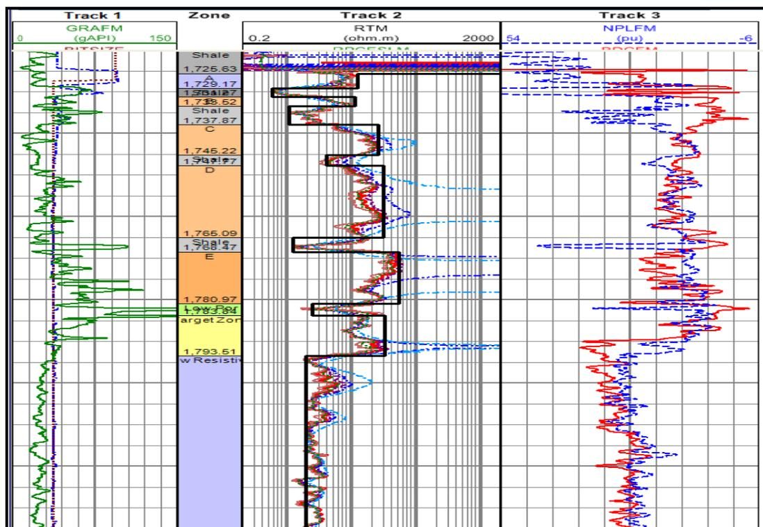
**Fig: 7.** Log of offset well with bed markers
