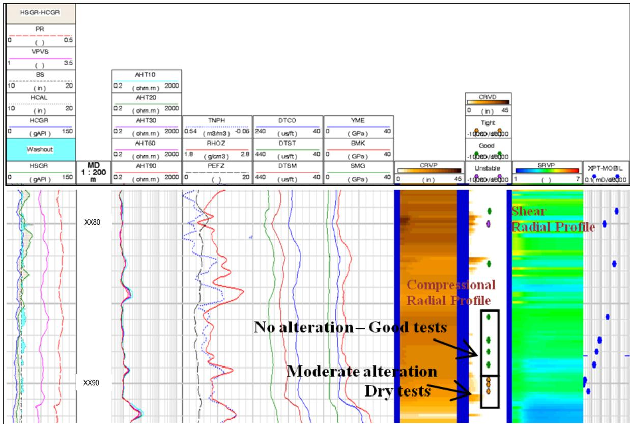
Fig 7. Integrated results of Monopole and Dipole radial profiling evaluation showing zones of formation alteration and formation tester measurement points.
