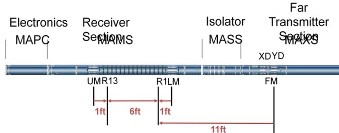
Fig 1. New generation Sonic tool configuration (Copyright © Schlumberger; Courtesy: Schlumberger Oilfield Review, 2006)
