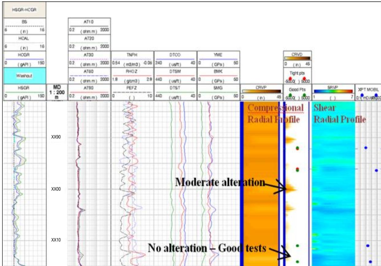
Fig 8. Integrated results of Monopole and Dipole radial profiling showing zones of formation alteration and formation tester measurements (Good tests) against zones of no alteration/ damage.
