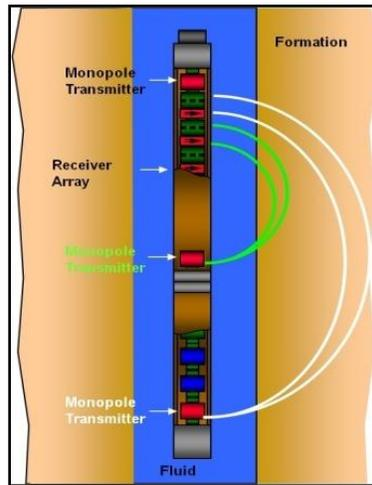
Fig 2. New generation sonic tool T-R spacing (Copyright © Schlumberger; Courtesy: Schlumberger Oilfield Review, 2006)
