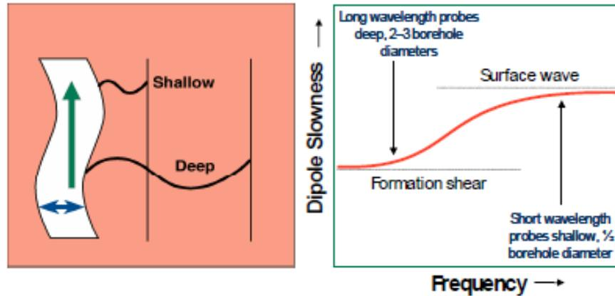
Fig 5. Dipole radial profiling principle (Jiang et al., 2008)
