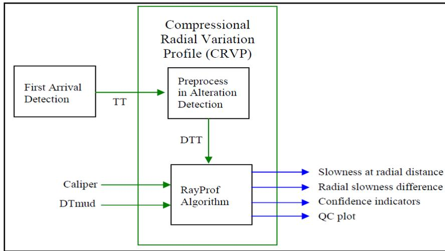
Fig 3. Compressional Radial Profiling schema
