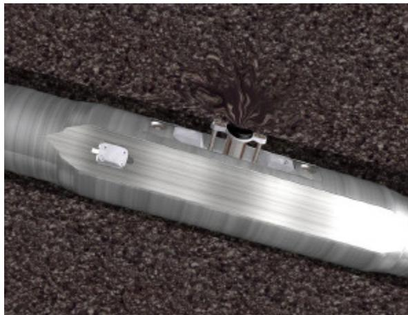
**Fig. 2. LWD formation pressure tester (TesTrak).**
