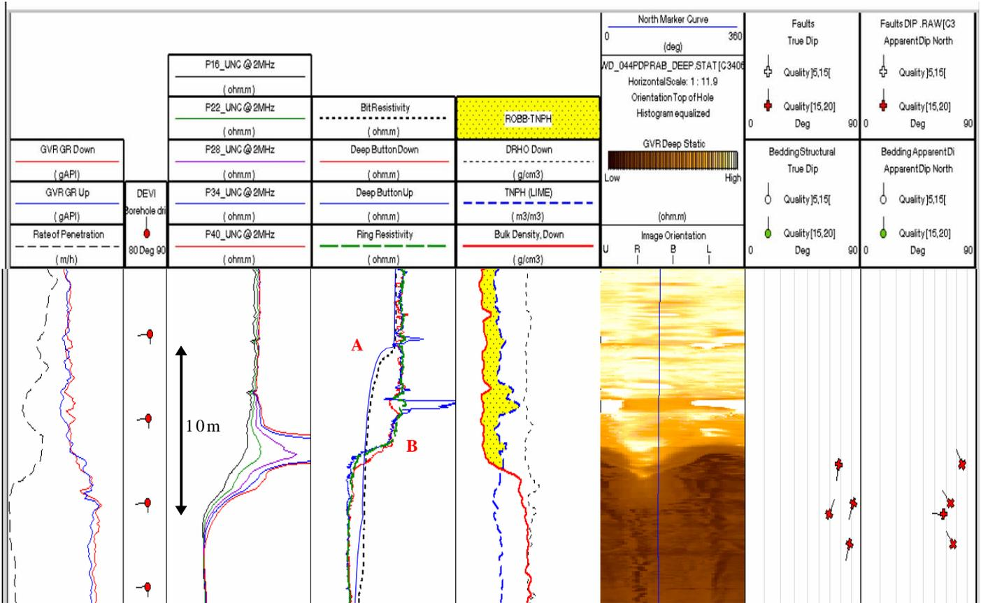
Figure 6: Magnification of figure 3: modeled bit resistivity curve (blue curve) superimposed on field bit resistivity curve (dotted curve). Blue curve modeled for bed resistivity contrast assuming no dip
