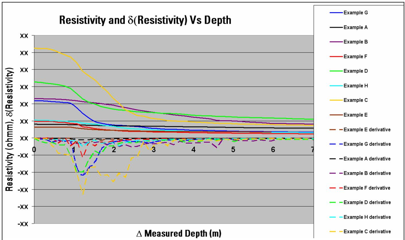
Figure 7: Graphic of bit resistivity (solid coloured lines) versus  $\Delta$  measured depth for 8 different examples. The dashed coloured lines represent the delta bit resistivity versus  $\Delta$  measured depth
