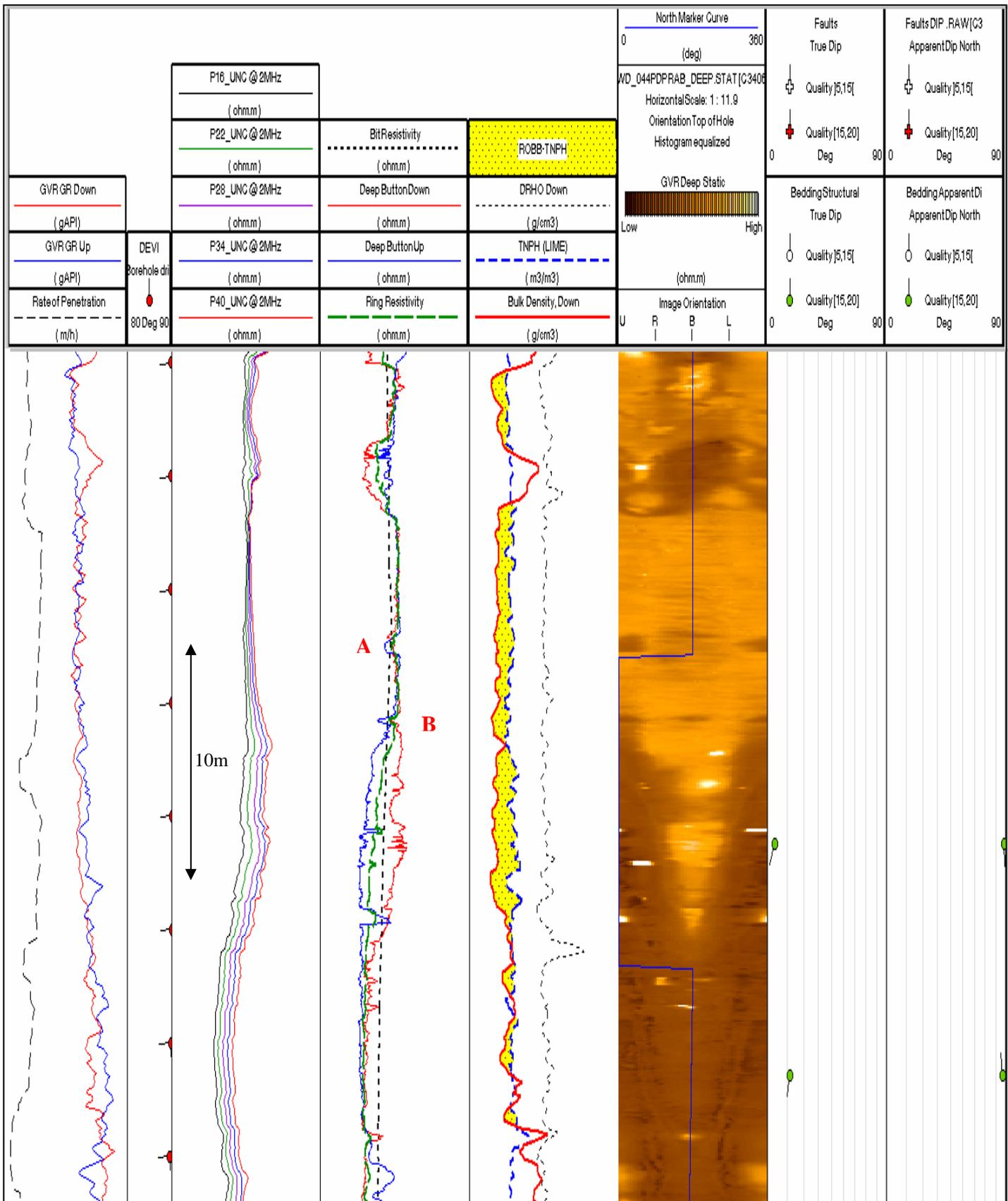
**Figure 2: Near horizontal wellbore crossing a bed with negligible structural dip. The bit resistivity detects the presence of a conductive bed with a point of inflexion at A. At point B the deep button up resistivity decreases while the deep button up remains high indicating the conductive bed is located above the wellbore**
