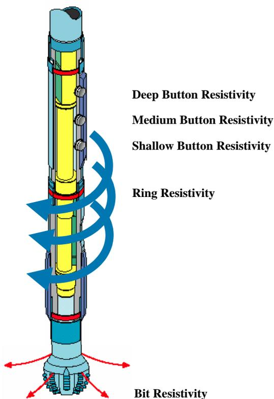
Figure 1: Schematic of GeoVision Laterolog-While-Drilling Resistivity Tool: button resistivity measurements are focused and azimuthal, the ring resistivity measurement is focused and non-azimuthal and the bit resistivity is non-focused non-azimuthal
