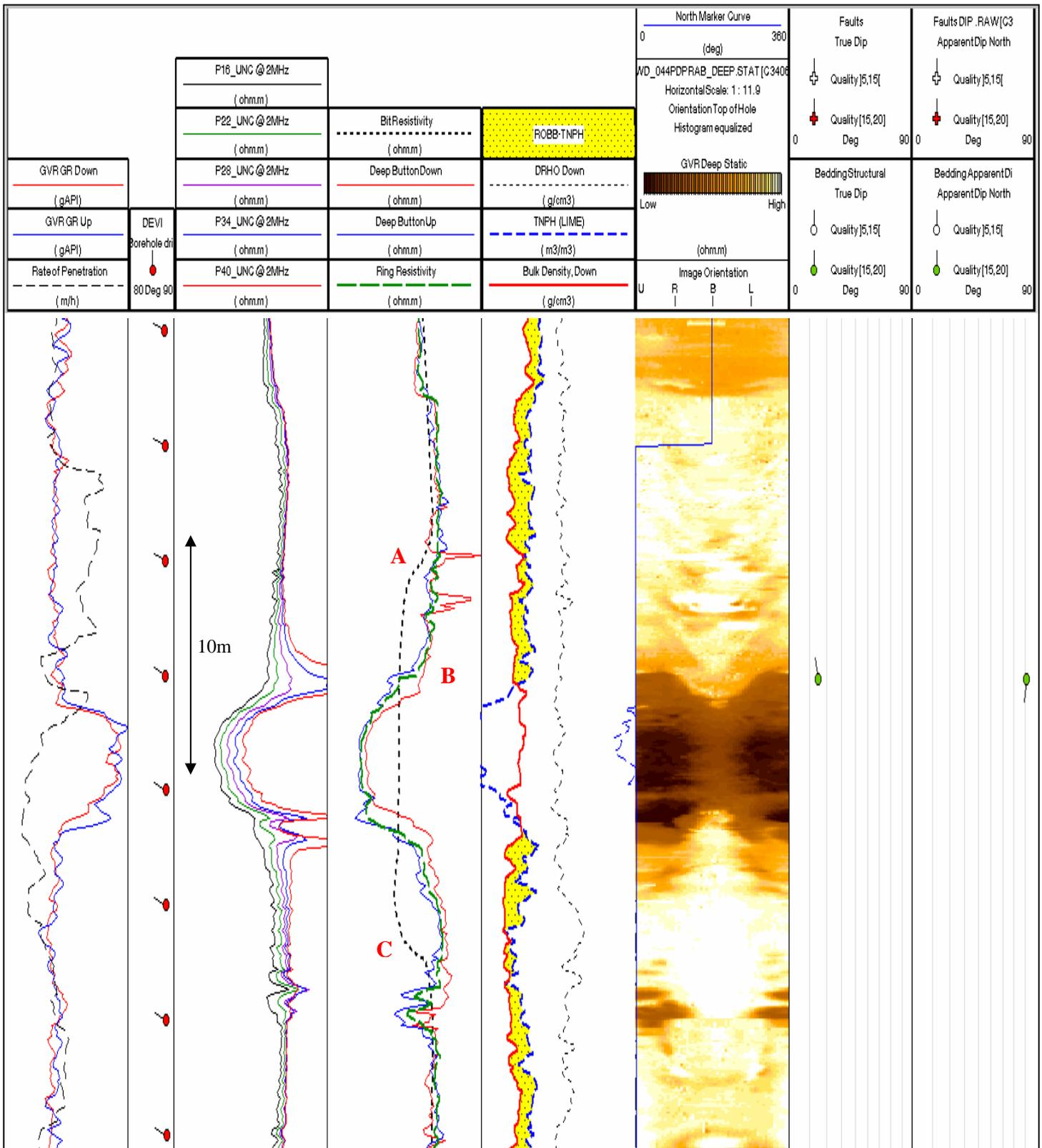
**Figure 4: Near horizontal well crossing a channel lens. The true structural dip of the feature is 15° and it is almost strike to the wellbore. The wellbore crosses the feature at high relative dip (82°) and this is consistent with the occurrence of a polarization horn (track 3). The bit resistivity curve (track 4) is sensitive to a conductive bed ahead of the bit since it begins to decrease at point A.**
