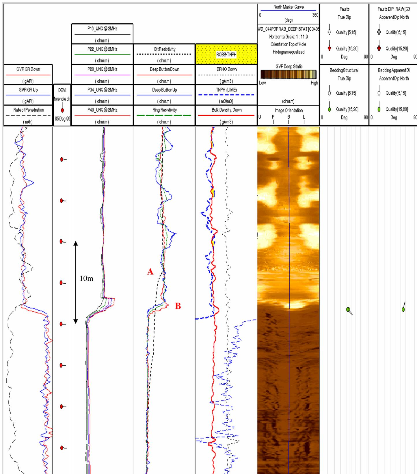
**Figure 5: Near horizontal wellbore crossing a shale channel whose true dip is 45° oriented south east. The bit resistivity first detects this channel at point A with a characteristic ‘concave’ behaviour. The button resistivity curves at point B confirm that the feature does not have zero apparent dip with the wellbore and that we are drilling up-dip**
