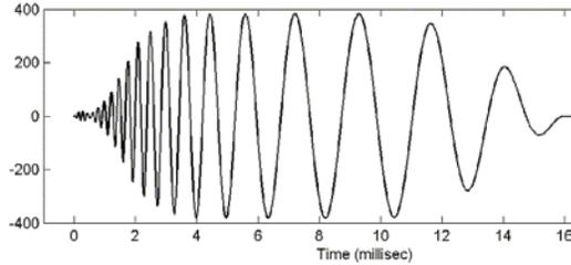
Fig. 2 Dipole Chirp Drive response.
