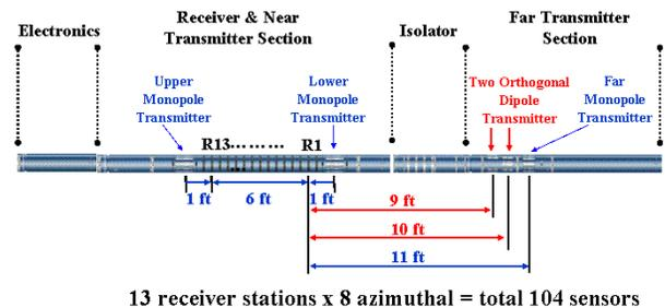
Fig. 1 New Sonic Acquisition Tool Geometry.
