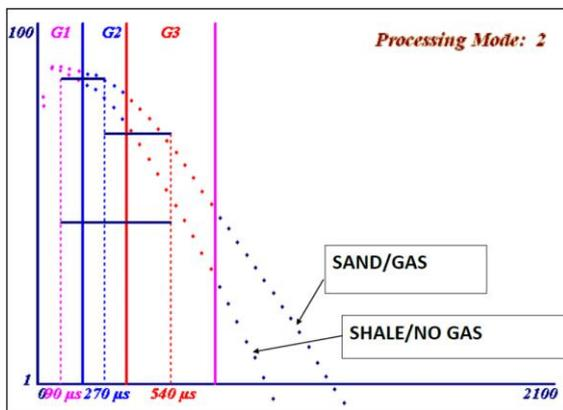
The fourth gas indicator comes from SGM2\_12 & SGM2\_23. These curves are mode two processed Sigma curves. They deflect in opposite directions due to different shape of the thermal neutron decay (convex or concave) in non gas and gas saturated formations.
