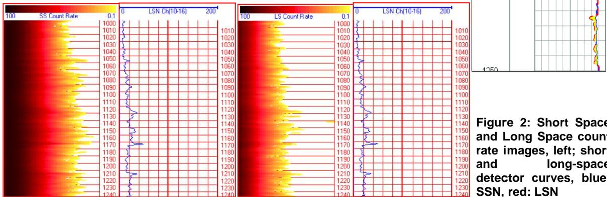
Figure 2: Short Space and Long Space count rate images, left; short and long-space detector curves, blue: SSN, red: LSN
