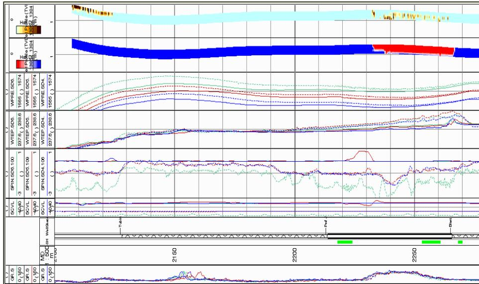
Figure 11: Shut-in Survey Data from Flagship\* tool string in Well 1
