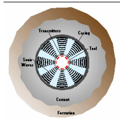
Fig-7 : Slim Cement Mapping Tool ; OD=1.875"; suitable for through tubing operations, Outputs standard 3ft CBL and 5ft VDL measurement in addition to radial continuous cement image (right)
