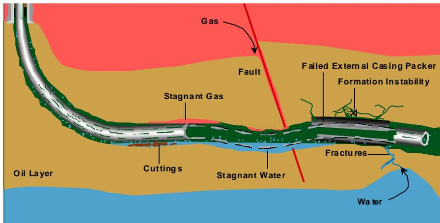
Figure-3: Potential problems in horizontal wells
