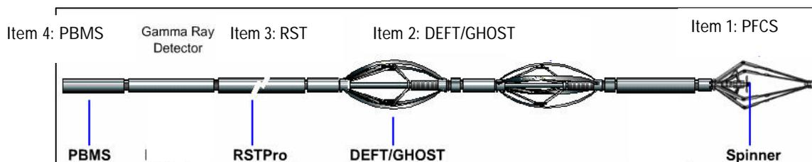
Fig-8: Schematic of Integrated Production logging tool string
