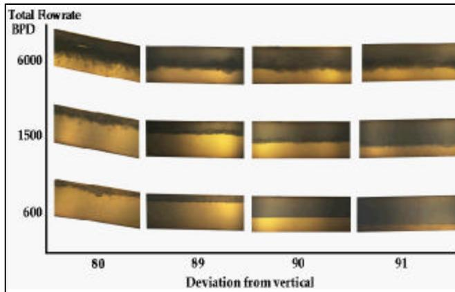
Fig-4: Effect of change in deviation on hold-up and fluid velocities; Water-Oil Stratified Flows in 5.5 in. Casing, Water Cut is 50%
