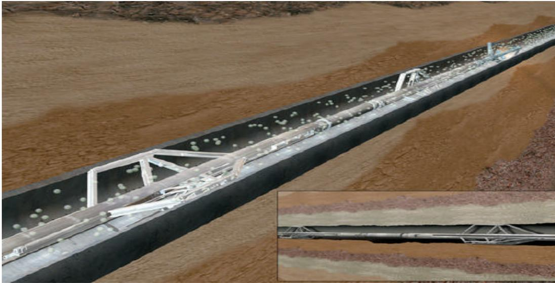
Fig-9: Wireline Tractor Schematic during Production logging and in Open hole (inset)
