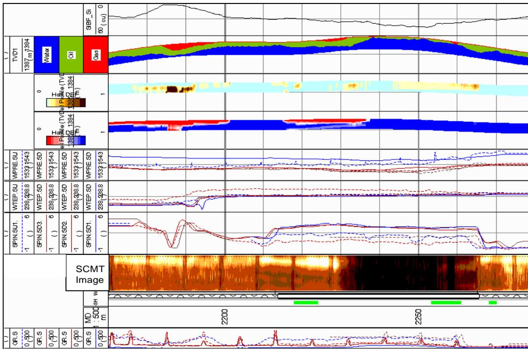
Figure 10: SCMT\* and Flowing Survey Data from Flagship\* tool string in Well 1
