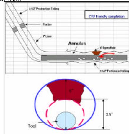
Fig-5: Changing flow ID due to shale sloughing / borehole collapse
