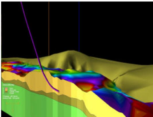
**Figure 4:** The 12¼" section is drilled into the reservoir: yellow represents the main HC-bearing sand. Anticipated gas is in the uppermost part of the reservoir.
