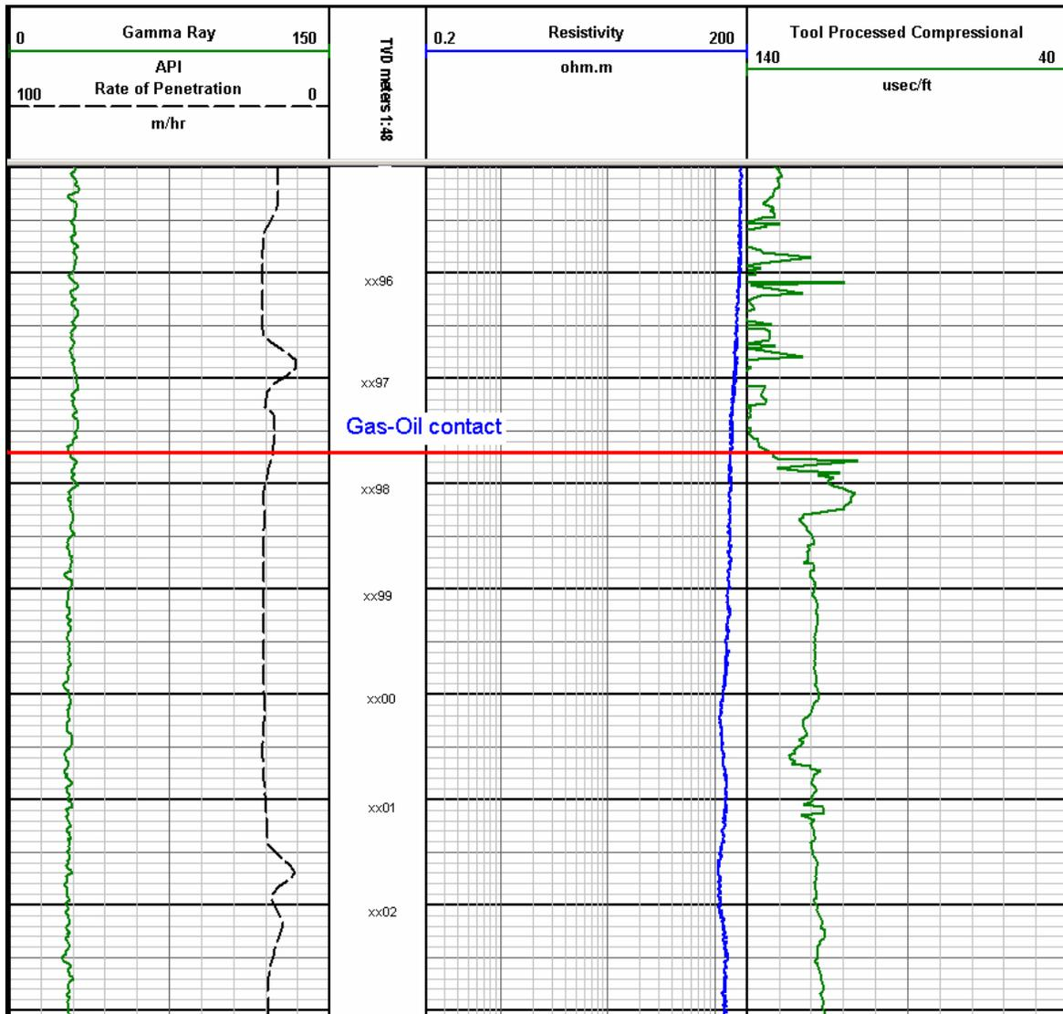
Figure 6: Tool-processed compressional slowness showing GOC.
