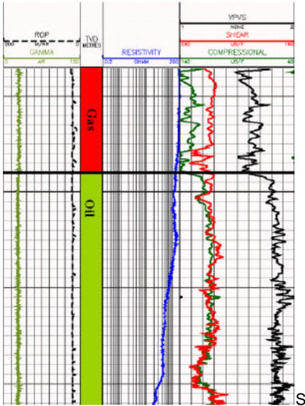
Figure 7: Post-processed compressional and shear slowness showing GOC.
