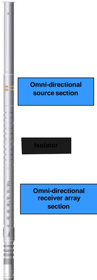
Figure 5: SoundTrak LWD acoustic tool elements
